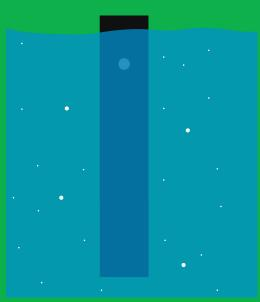
The entire conducting area must be submerged in order to get accurate readings.
