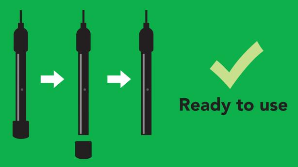
Be sure to watch out for air bubbles, as they can get caught inside the probe housing and throw off your results. Lightly tap your conductivity probe to knock out any bubbles caught in the probe.
