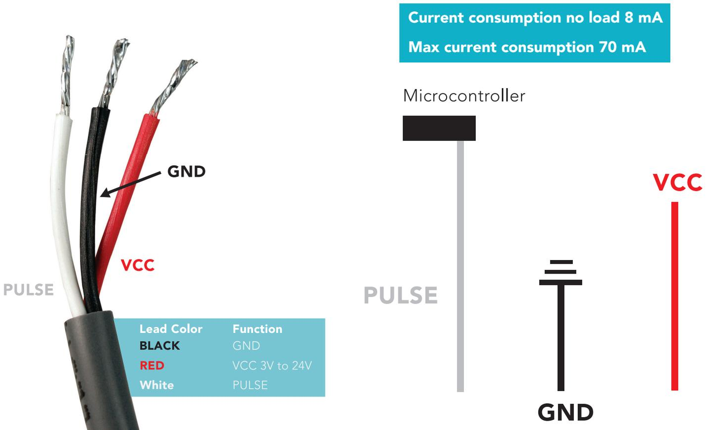
**REVERSING THE POLARITY WILL DESTROY THE FLOW METER**
