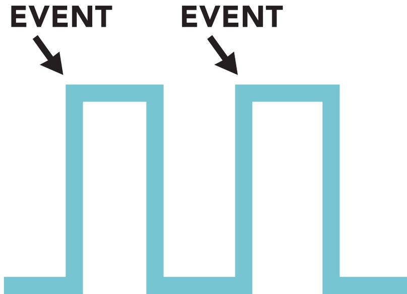
The amount of liquid moving through the flow meter is quantified by the frequency that the flow meter outputs. This is known as the flow meters K-factor.
